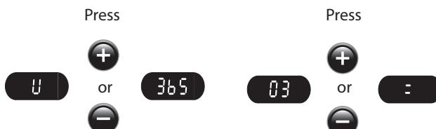
If a "U" is displayed on the LED screen, by pressing the Pump 1 button the sanitising system will switch from "U" to "O3", after which you will exit the programming menu.
