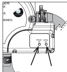
**Note:** the CLEARRAY system only works when the jets pump 1 is operating at reduced speed (filtration, etc.).
