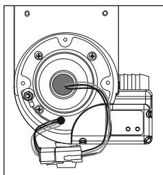
**3-** Disconnect the UV lamp connector (6) from the power supply (4).
